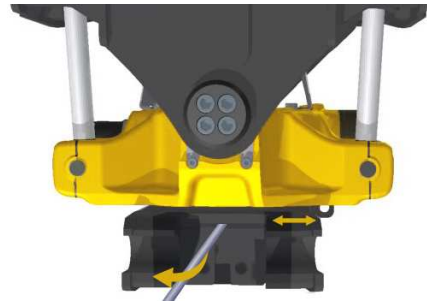
Figure 35. Rotate the quick coupler to the left.
